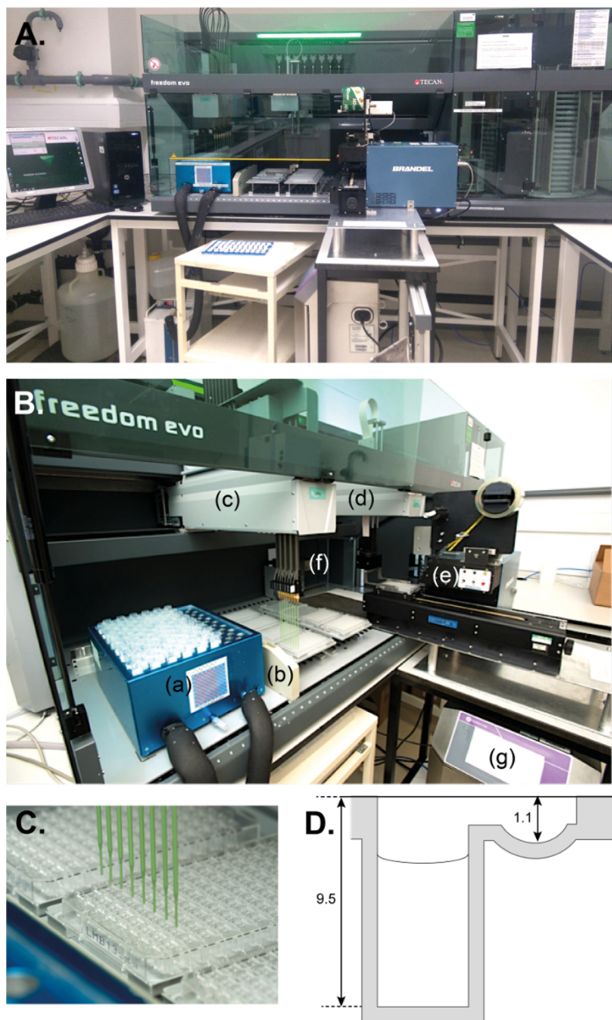
Figure 1: Filling the reservoirs with initial screening kits. (A) Overview of the fully automated system 1. The carousel is a separate automated unit with plate stacks and it is housed in a well made of clear acrylic sheets on the right-hand side the main deck. (B) The main deck of the liquid handler in operation with (a) the tube-cooling carrier (connected to a chilling unit underneath, not shown), (b) the fast wash station (connected to drainage, not shown), (c) the pipetting arm filling 8 reservoirs of a 96-well crystallization plate, (d) the gripper arm bringing a filled plate onto (e) the motorized SBS carrier of the plate sealer. In the back of the deck is (f) the printing head of the inkjet printer connected to (g) the inkjet control unit underneath the sealer. (C) A labeled plate (name of the screen and date of production) being filled with crystallization conditions by 8 conductive fixed tips made of Polytetrafluoroethylene-coated stainless steel. (D) Cross-section of a sealed crystallization well. The reservoir contains 80 \mu L of crystallization condition (while the upper well is empty). Reservoir and upper-well depth specifications are in millimeters. Please click here to view a larger version of this figure.
