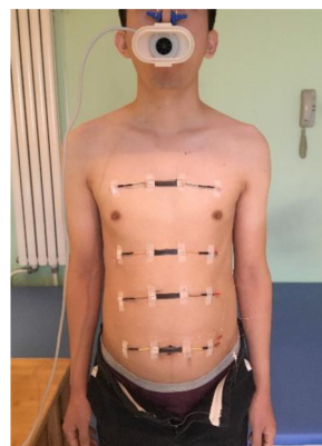
Fig. 1. Respiration measurement using wearable strain sensor (WSS) and spirometer.
