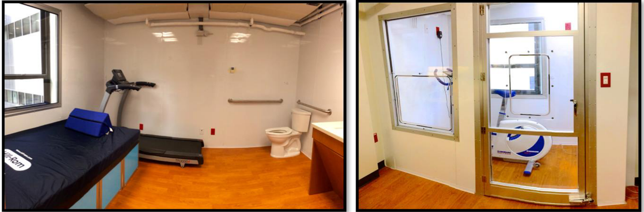
Fig 1. VCU metabolic chambers. Left: big chamber as a living room; right: small chamber (flex room) for single activities. Boxes can be added to the small chamber for resting energy expenditure studies.
