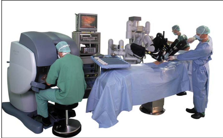
FIGURE 1. The daVinci ® robotic system: surgical console, vision cart, and patient-side surgical cart. Photo courtesy of Intuitive Surgical, Sunnyvale, CA.
