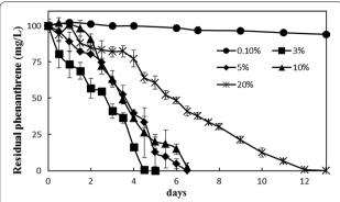
**Fig. 1** Effect of salinity on phenanthrene degradation by halophilic consortium CY-1. Consortium was cultivated batch-wise (second round) in SSDM under 0.1, 3, 5, 10 and 20% (w/w) salinity at 30 °C, 150 rpm. Samples were collected in the degradation process from day 1 to day 13
