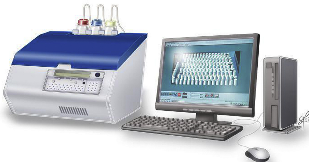
Fig. 1 External view of the luminometer connected to the monitor for real-time display of ROS production on the monitor screen.
