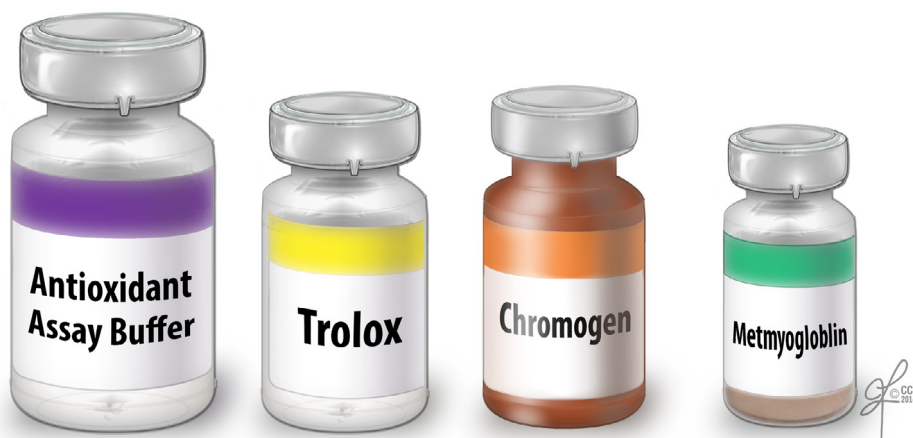
Fig. 4 Components of the TAC kit used in colorimetric measurement of total antioxidants. It comprises a standard assay buffer, Trolox standard, chromogen, and metmyoglobin.
