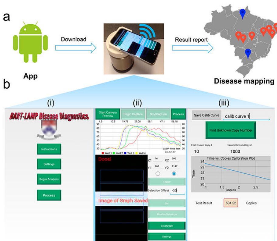
Figure 2. Android App for the smartphone-based molecular detection and disease mapping. (a) A flowchart of the SCC-based molecular detection and disease mapping. Red and blue dots denote, respectively, locations of positive and negative tests. (b) Screenshots of our smartphone interface: (i) main menu, (ii) real-time monitoring of the reactors of the MIAR chip, and (iii) calibration curve and result report.
