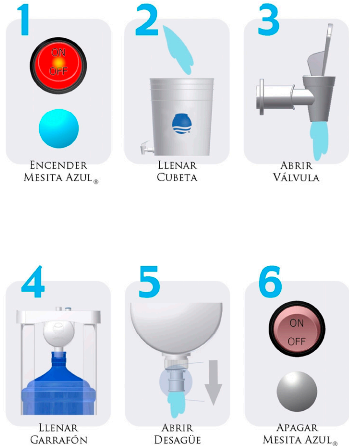
FIGURE 1. The Mesita Azul system includes a bucket for source water, the ultraviolet disinfection chamber, a safe storage container ( garrafon ) for treated water, and instructions for correct use. This figure appears in color at www.ajtmh.org .
