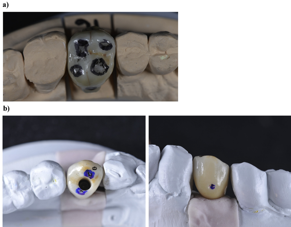
Fig. 4. Glazed crowns after try-in and landmarking of areas to be ex vivo analysed. a) Final crown on tooth #16. Landmarking of areas to be analysed: occlusal contact points and control areas on buccal and palatal faces, which are located up to the undercut created to remove the crown. b) Screw-retained crown on implant (tooth #34). Landmarking of areas to be analysed: occlusal contact points and control areas on buccal and lingual faces, which are located up to a small groove performed in the restoration surface.
