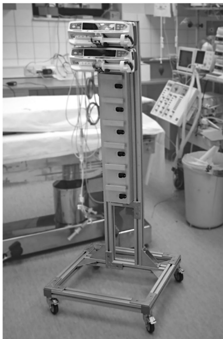
Fig. 3 Prototype closed-loop hemodynamic stabilization system, with two (out of eight possible) computer controlled infusion pumps attached. Connectors for blood pressure transducers and user interface PC are situated on the backside of the column
