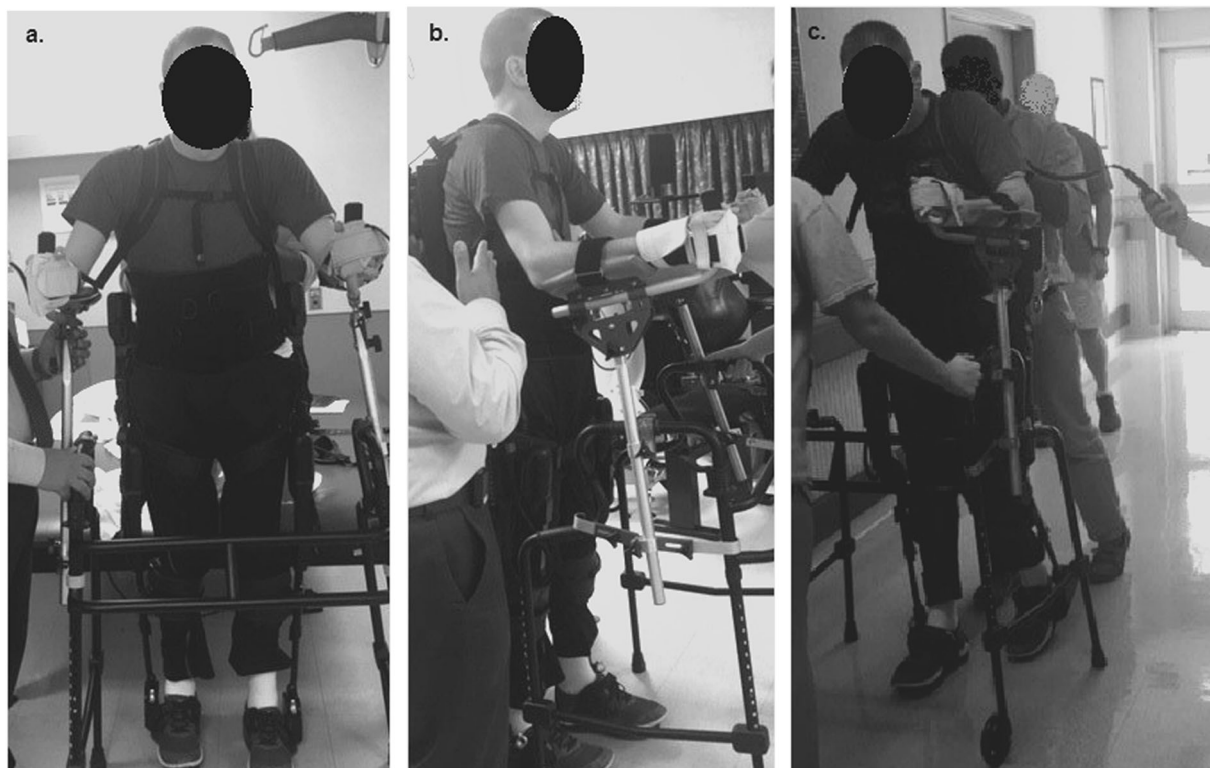
Fig. 1 a Frontal view of subject standing upright in exoskeleton device using rolling platform walker. b Lateral view of device setup, showing hand splints used to cuff the participant's hands to the platform
