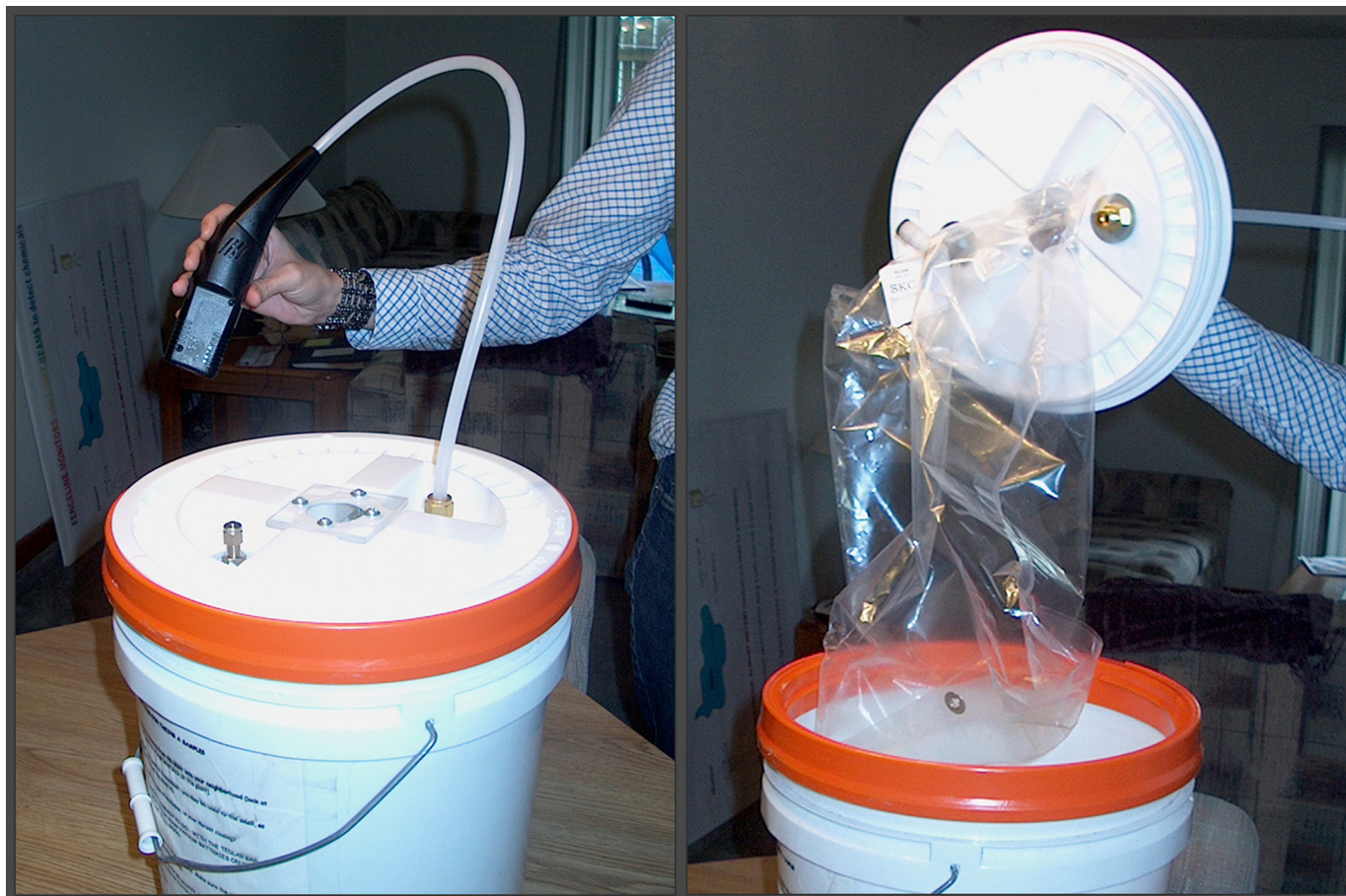
An early bucket sampler used by the Louisiana Bucket Brigade employed a hand-held vacuum cleaner to pump the air out of a five-gallon plastic container, then draw ambient air into through a stainless steel inlet to a nonreactive plastic bag. Image: © Gwen Ottinger/Drexel University.
