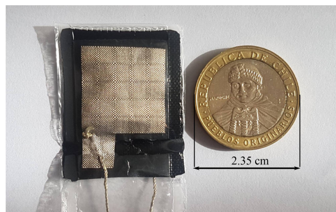
Figure 3. Top view with dimensions of the resistive textile pressure sensor.
