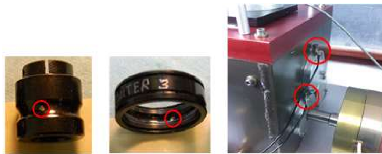
Figure 15. The IRF and ORF rolling bearings, and two sensors of one side.
