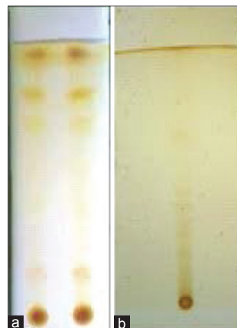
Figure 1: (a) Thin-layer chromatography fingerprint (R f = 0.69 and 0.71) of karanjin in Ethanol: ethyl acetate (16:4 v/v) and Ethyl acetate: methanol: distilled water (10:3:7) solvent system, (b) Thin-layer chromatography fingerprint of Embelin (R f = 0.36) in N-propanol: butanol: ammonia (11: 3:6) solvent system
