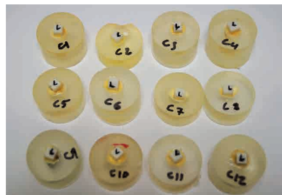
Fig. 2: Ceramic cubes of lithium disilicate and zirconia ceramics
