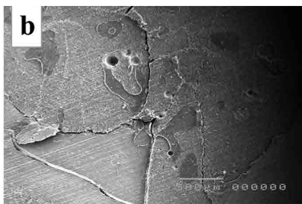
Fig. 5: SEM images of fracture mode. Lithium disilicate: (a) irradiated surface (b) non-irradiated surface.
