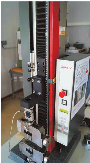
Fig. 3: Universal testing machine (Zwick 2.5kN, Germany)
