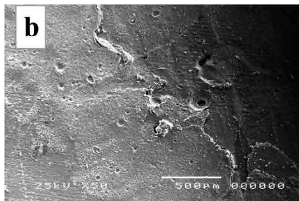
Fig. 6: SEM images of fracture mode. Zirconia: (a) irradiated surface (b) non-irradiated surface.
