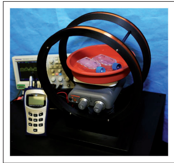
Figure 1. ELF-EMF Emitting Device Setup. EMF Emitting Device Is an 11" Diameter Helmholtz Coil Equipped With a Warm Bath Heated With Ceramic Heating Element to Maintain 37°C Constant Temperature. Oscilloscope Is Used to Measure Frequency. Gauss Meter Is Used to Measure Field Strength.
