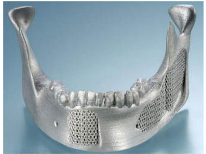
Figure 3. Selective laser melting is capable of rapid prototyping metal-based models including patient specific anatomy.
