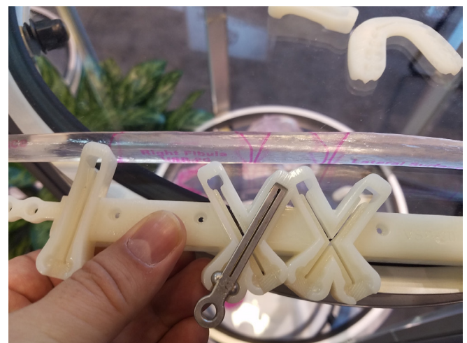
Figure 8. A 3D printed cutting jig designed for guided osteotomies of a free fibula that will then be used from mandibular reconstruction (Embodi 3D, Biomedical 3D printing community).
