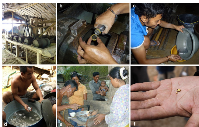
Figure 2. Liquid mercury is used in artisanal and small-scale gold mining. a) Trommels are used to crush rock and mix mercury with ore. b) As much as 1 kg of liquid mercury is added to each trommel along with water and 20 kg of ore. c) Excess mercury is recovered, but mercury-rich mine tailings are often released directly into the environment. d) Additional mercury is used on the mercury–gold concentrate to form a solid amalgam, which may be isolated by hand. e) The mercury–gold amalgam is heated with a torch to distill the mercury and allow isolation of gold. f) A sample of gold isolated in an artisanal mine. All images are used with permission from Yayasan Tambuhak Sinta (YTS) and Pure Earth.
