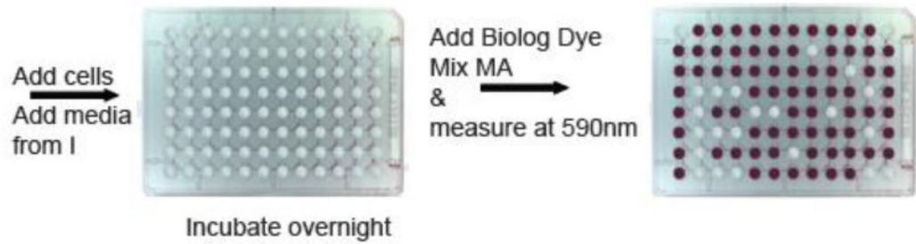
Figure 2. Workflow for a customized Biolog assay set up (96-well plate picture courtesy of Biolog Inc.)
