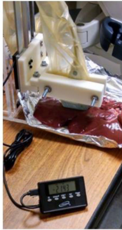
Figure 1. Measured distance calibration on the GE Logiq E9 (9 MHz probe) for determination of ex vivo ground-truth speed of sound values.
