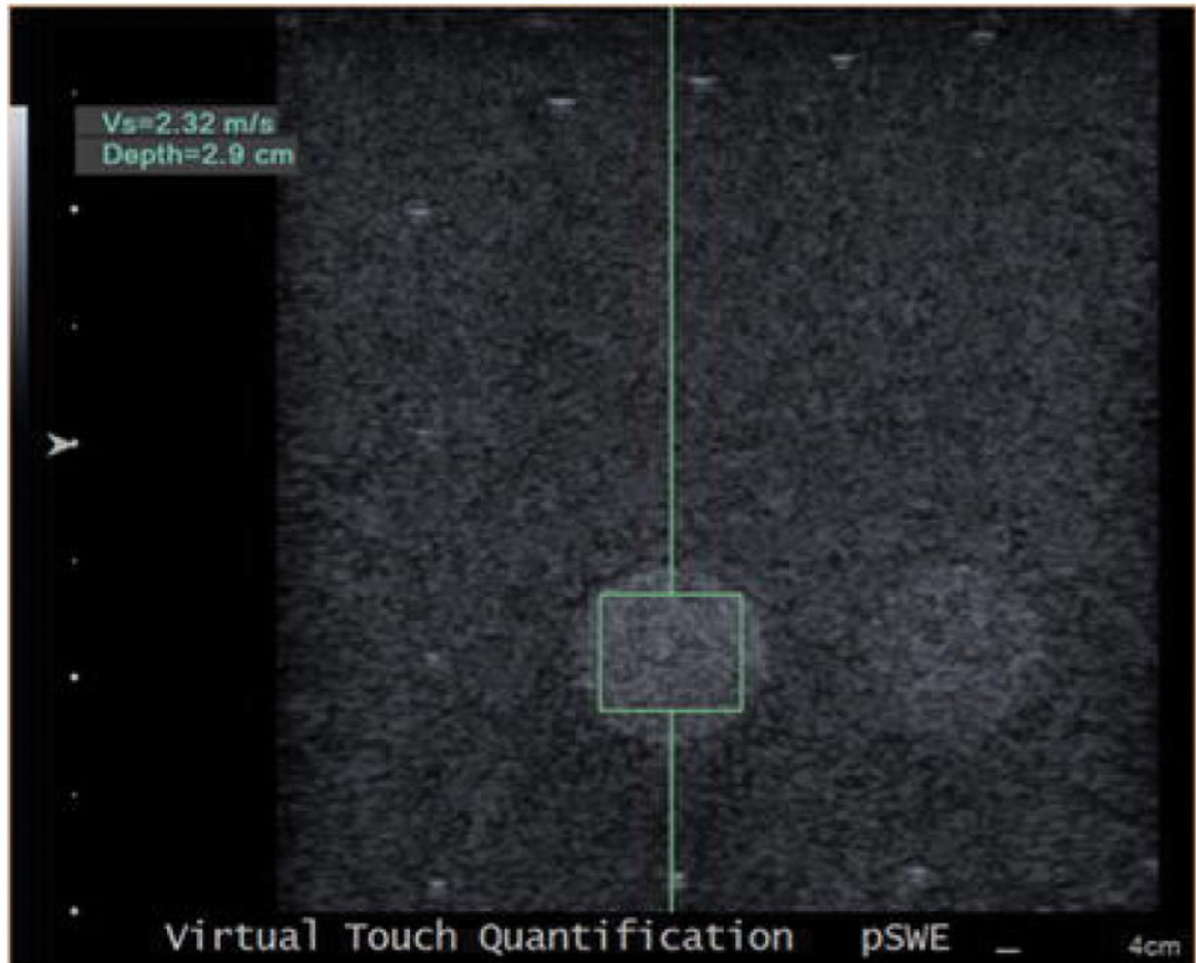
Figure 3. pSWE acquisition on a phantom. Green box is the focus of ARFI excitation. Shear wave speed value is indicated in left panel.
