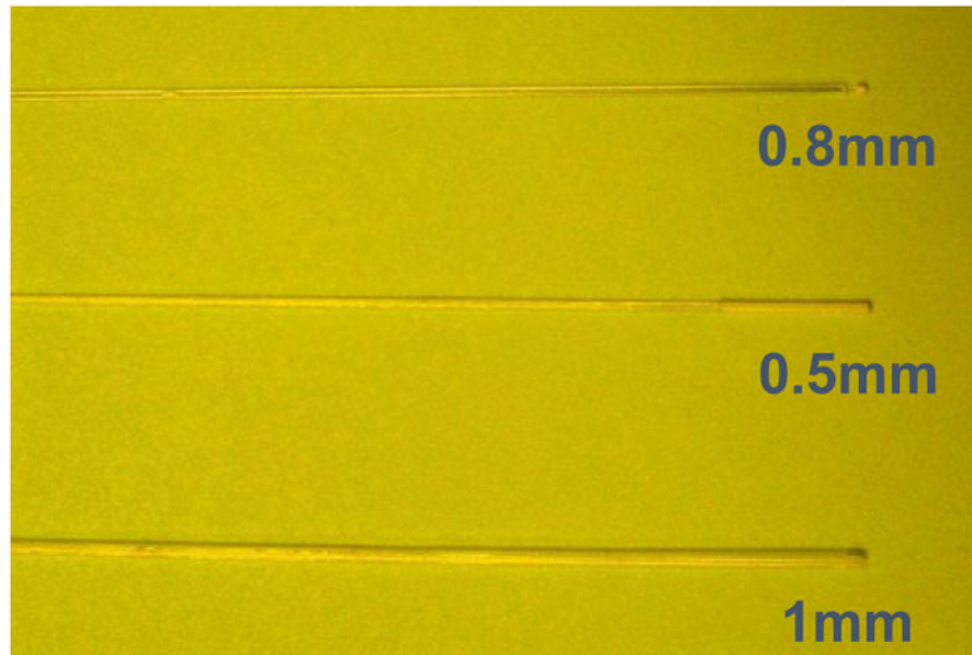
Figure 6. Picture of the three isotropic detectors used in the study. (a) Cardiofocus with 1mm tip, (b) Cardiofocus with 0.5mm tip and (c) Medlight with 0.8mm tip.
