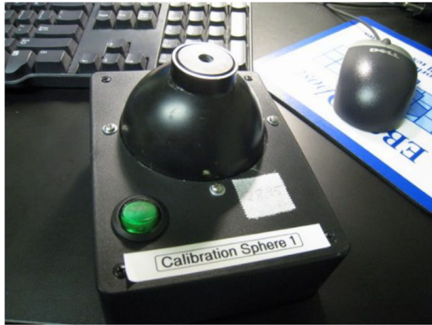
Figure 4. Picture of the light-emitting diode (LED) light source.
