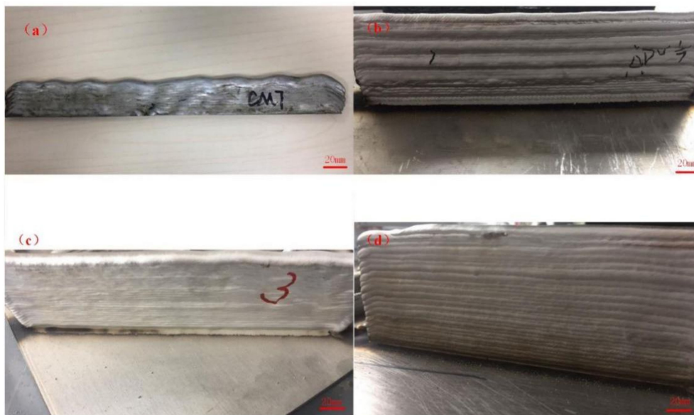
Figure 4. The multilayer additively manufactured 2219 aluminum wall samples using different arc modes: (a) CMT; (b) CMT-ADV; (c) CMT-P, and (d) CMT-PADV.
