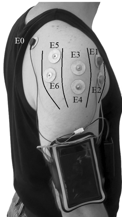
Fig. 1 Deltoid sections and surface electrode placement E0, ground; E1/E2, anterior deltoid; E3/E4, middle deltoid; E5/E6, posterior deltoid
