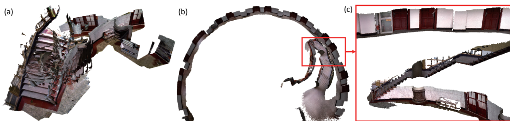
Figure 10. Reconstruction results of an arched department. (a) is produced by BundleFusion [33]. The system failed and gave an unsatisfactory result. (b) is produced by our system. (c) gives surface details on the stairs.
