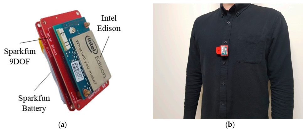
Figure 2. Overview of the apparatus. (a) Packaging of the Intel Edison, Sparkfun 9DOF, and Sparkfun Battery; (b) Appearance of the apparatus when worn by participant.
