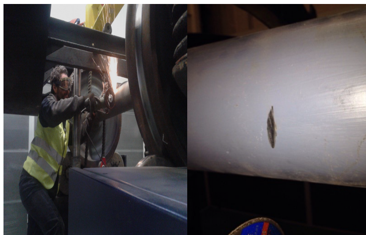
Figure 6. Inducing defects and result of Defect N1.
