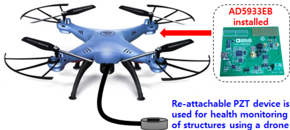
Figure 7. Drone electromechanical (EMI) technique concept [110].
