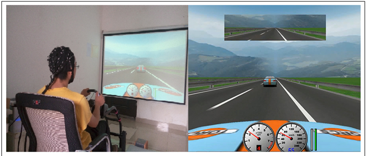
Fig 2. Driving simulator (left) and TORCS-based [35] driving scenarios (right). The participant in Fig 2 has given written informed consent (as outlined in PLOS consent form) to publish these case details.
