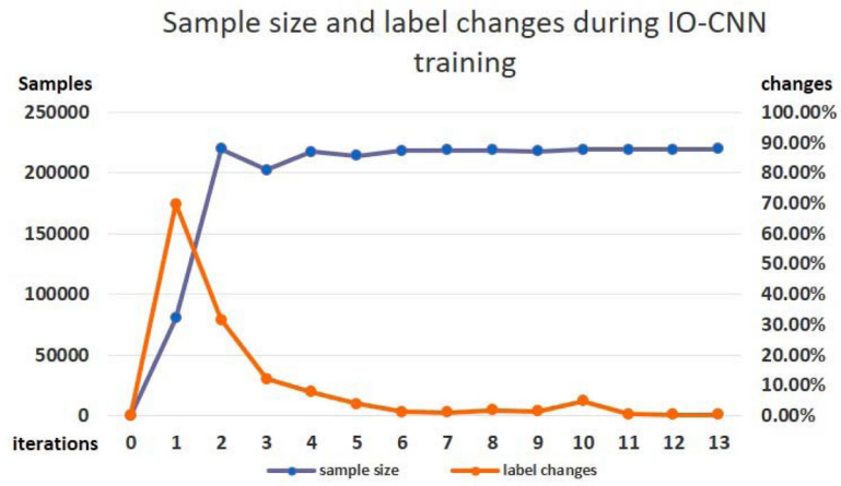
Fig. 7. Sample size's dynamic changes and label change percentages during IO-CNN training. Iteration 0 is the weak label initialization process, where IO-CNN is not trained yet. Initial labels (80,293 initial training samples) were first used in iteration 1 for IO-CNN training.
