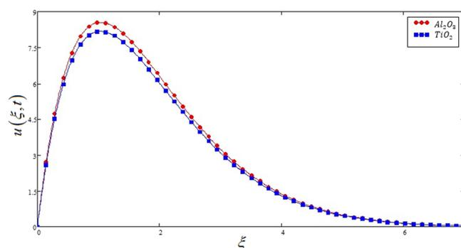
**Figure 11.** Comparison of velocities profiles of  $Al_2O_3$  and  $TiO_2$  for Casson nanofluids when  $Pr=0.71$ ,  $Gr=10$ ,  $Nr=2$ ,  $\varphi=0.04$  and  $t=1$ .
