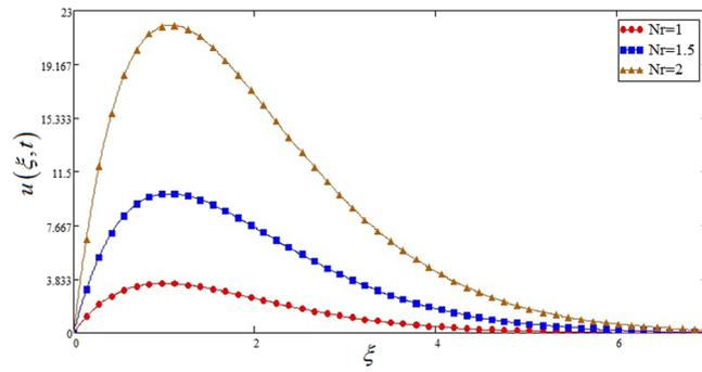
**Figure 8.** Effects of radiation parameter  $Nr$  for  $TiO_2$  on the velocity profile of Sodium alginate based nano fluid when  $Pr=0.7$ ,  $Gr=8$ ,  $\varphi=0.04$  and  $t=1$ .
