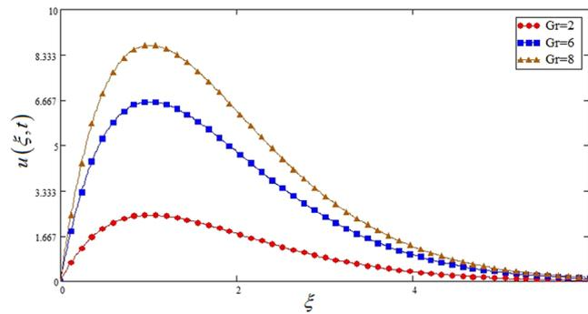
**Figure 5.** Effects of thermal Grashof number  $Gr$  on the velocity profile of Sodium alginate based Casson nano fluid when  $Pr = 0.7$ ,  $Nr = 2$ ,  $\varphi = 0.04$  and  $t = 1$ .
