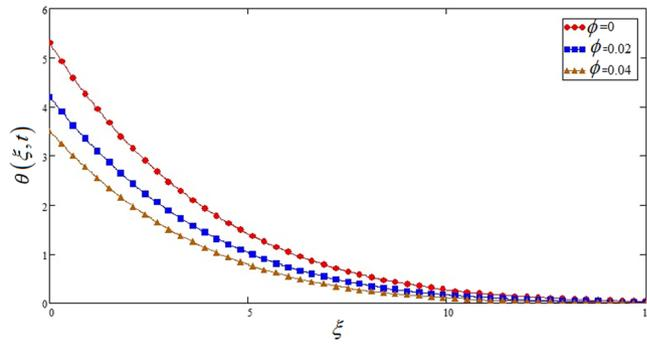
**Figure 4.** Effects of nano particles volume fraction parameter  $\varphi$  on the temperature profile of Sodium alginate based nano fluid when  $Pr = 5$  and  $t = 1$ .
