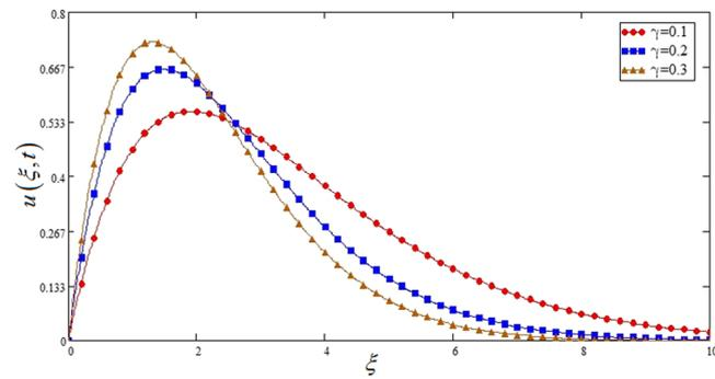
**Figure 2.** Effects of Casson fluid parameter  $\gamma$  on the velocity profile of Sodium alginate based Casson nanofluid when  $Pr = 0.7$ ,  $Gr = 2$  and  $\varphi = 0.04$ .
