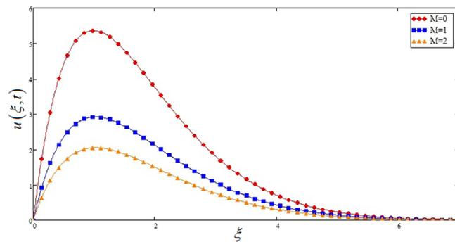
**Figure 6.** Effects of magnetic parameter  $M$  on the velocity profile of Sodium alginate based Casson nano fluid when  $Pr = 0.7$ ,  $Nr = 2$ ,  $Gr = 10$ ,  $k = 2$  and  $t = 1$ .
