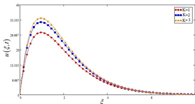
**Figure 7.** Effects of permeability of porous medium  $k$  on the velocity profile of Sodium alginate based nano fluid when  $Pr = 10$ ,  $Gr = 10$ ,  $Nr = 8$ ,  $\varphi = 0.04$  and  $t = 1$ .
