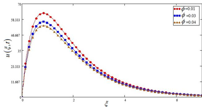
**Figure 3.** Effects of nano particles volume fraction parameter  $\varphi$  on the velocity profile of Sodium alginate based nano fluid when  $Gr = 0.2$ ,  $Nr = 0.2$  and  $t = 1$ .
