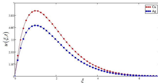
**Figure 10.** Comparison of velocities profiles of  $Cu$  and  $Ag$  Casson nanofluids when  $Pr=0.71$ ,  $Gr=10$ ,  $Nr=2$ ,  $\varphi=0.04$  and  $t=1$ .
