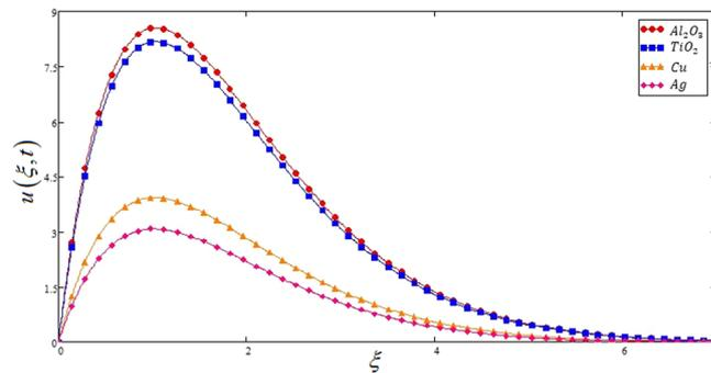
**Figure 9.** Comparison of velocities profiles for different types of nano particles for Casson nanofluids when  $Pr=0.71$ ,  $Gr=10$ ,  $Nr=2$ ,  $\varphi=0.04$  and  $t=1$ .
