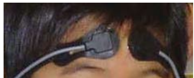
FIGURE 2 Placement of near-infrared spectroscopy (NIRS) probes. The probes of a two-channel NIRS apparatus (NIRO200, Hamamatsu Photonics, Inc.) were placed bilaterally on the subject’s forehead to enable the measurement of \Delta\text{oxy-Hb} and \Delta\text{deoxy-Hb} in the bilateral frontopolar prefrontal cortex
