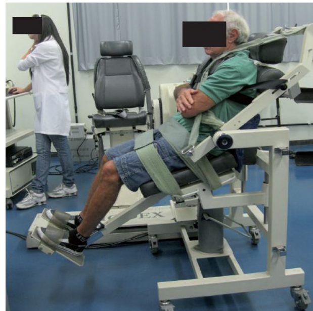
Figure 1 Positioning of a subject on the Biodex ® isokinetic dynamometer to test flexor & extensor trunk flexor & extensor concentric muscle strength.
