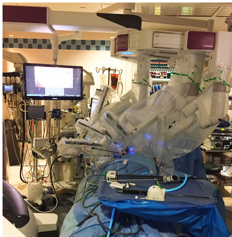
Figure 3 The da Vinci Xi ® has a boom-mounted system, which enables the surgical cart to be placed at any position around the patient.
