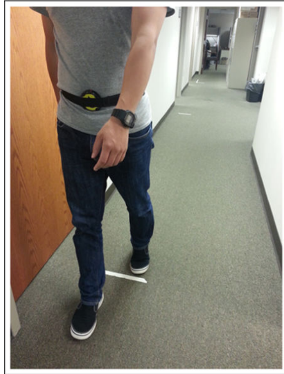
Figure 7. Subject walking on a 12-m walking pass with eButton strapped at lower abdomen.
