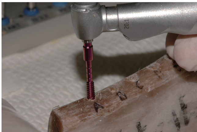
Fig. 1. The probe used to measure the bone density of the bone specimen. The probe has an inverse cone shape, allowing the torque measurement needed to win the friction exerted on the bone wall by its first thread. The average of all torque instantaneous torque values measured throughout its descent, Cm, has been showed to be a reliable measurement of bone density.
