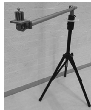
Fig. 1 Reference frame with 500 g weight used for performing the reaching tasks
