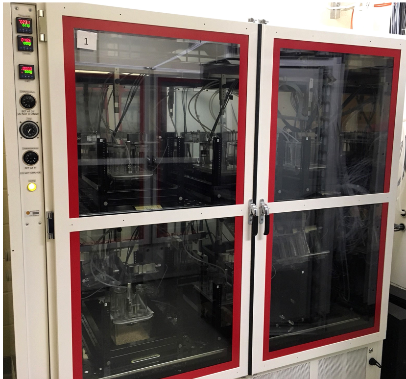
Figure 1. The PhenoMaster TSE system. One climate chamber can harbor 6 boxes that can measure O 2 , CO 2 , food intake, water consumption.
