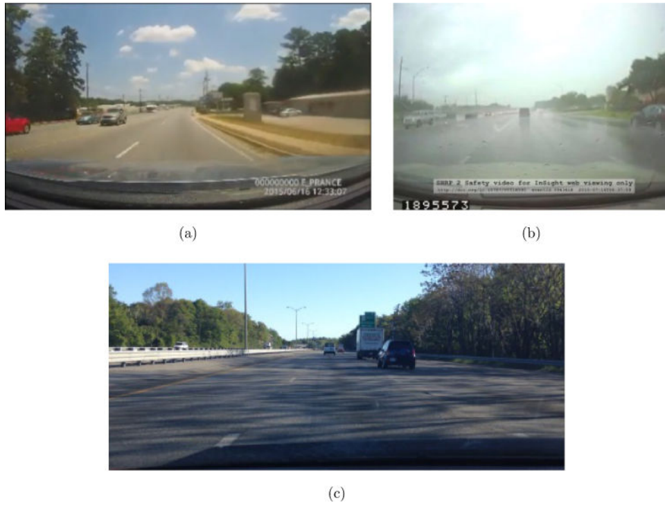
Fig. 1. Lane markers with weak signals. (a) An image with high resolution 1604 \times 768 captured by the E-PRANCE EP503 vehicle camera. 13 (b) A frame with resolution 480 \times 360 from SHRP2 study. 38 (c) An image with high resolution 1604 \times 768 but weak lane-marker signal.
