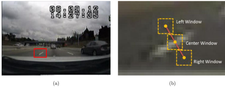
Fig. 6. Illustration of conjugate windows. (a) A naturalistic driving image. (b) Magnification of the marked area in (a), with a pair of conjugate windows and a center window. The red line in (b) connects the centers of the left window and the right window, perpendicularly to the direction of the lane marker, and the centers of the window lie on the lane marker (color online).
