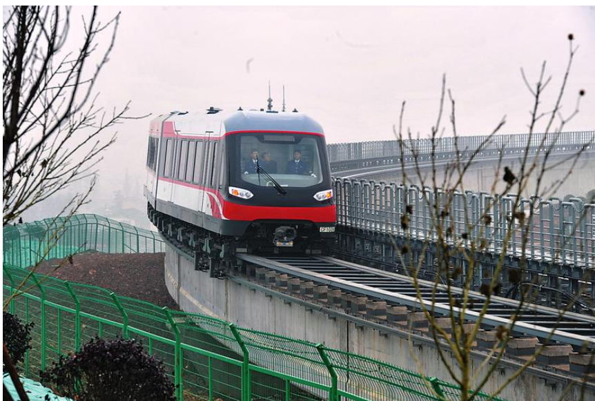
Figure 1. Changsha Maglev Express train in a small-radius circle.
