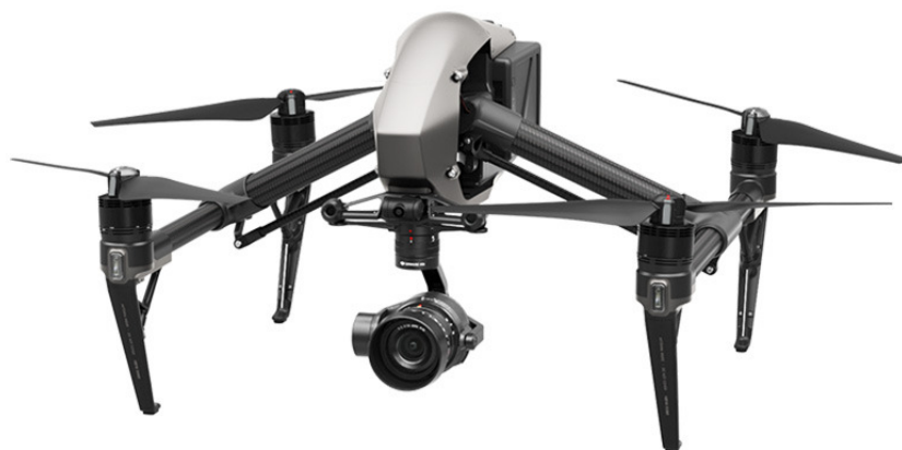
Figure 3. Inspire 2 with Zenmuse X5S for crack identification.
