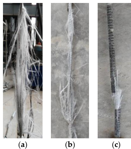
Figure 2. Failure modes of GFRP bars under cyclic load: (a) form of blasting damage; (b) form of splitting damage; and (c) form of fracture failure.
