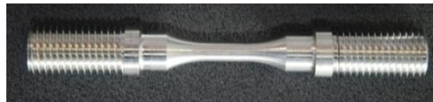
Figure 1. Sample used in monotonic tensile and creep tests.
