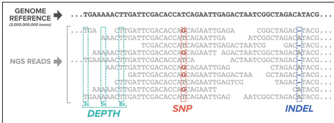
Figure 2. Next-generation sequencing reads aligned to a reference genome demonstrate two mutation types: a single-nucleotide polymorphism where a guanine has replaced a thymine and, further downstream, a deletion of an adenine. Depth of coverage of 3 \times , 5 \times , and 8 \times indicates the number of reads at each position. This image was adapted from figure 2 in Muzzey, Evans, and Lieber (2015). It is licensed under Creative Commons Attribution 4.0 International License ( http://creativecommons.org/licenses/by/4.0/ ). Modifications were made to include only a portion of the original image.
