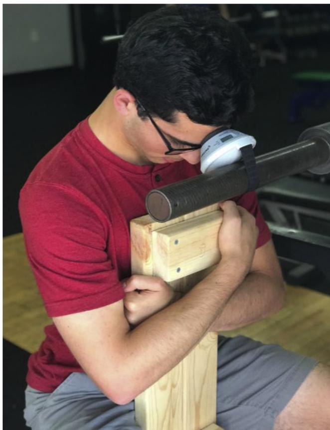
Fig. 1. Image of flexion strength being measured using the MicroFet2 dynamometer and custom built seat.
