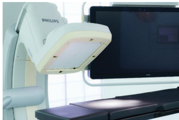
Figure 1. The navigation system consists of a surgical table digitally integrated with a ceiling-mounted motorized C-arm with 2D/3D imaging capabilities and a medical grade monitor where intraoperative imaging is superimposed with the camera images (cf. Figure 2). Note that the cameras are integrated at the middle of each side of the detector housing.
