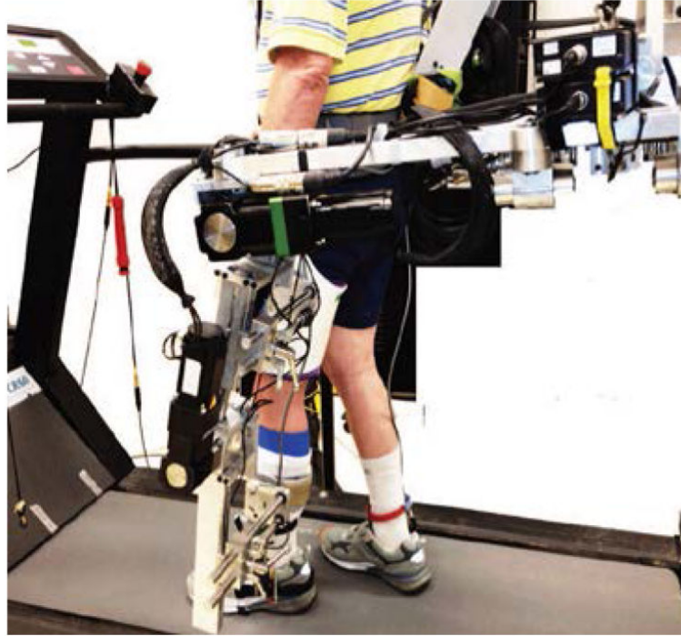
Fig. 1. The active leg exoskeleton (ALEX) worn by the subjects on their affected extremity during training and treadmill evaluation.
