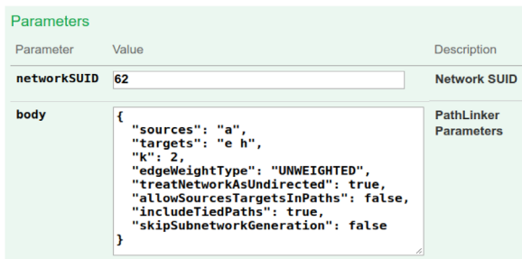
(b) API parameters for PATHLINKER in JSON format in the Swagger user interface.
