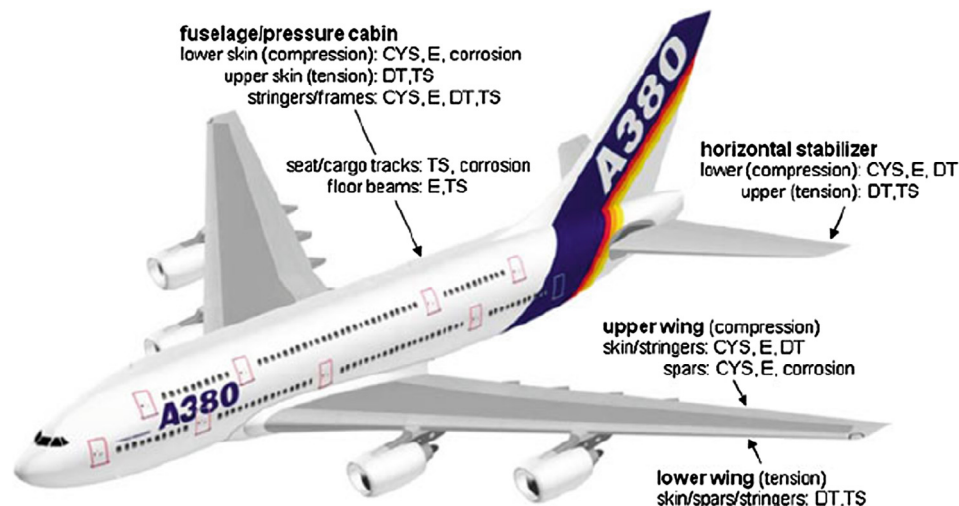
Fig. 1. Engineering properties needed for transport aircraft, where: FAT = Fatigue; FT = Fracture Toughness; FCG = Fatigue Crack Growth (FAT, FT and FCG are denoted as Damage Tolerance (DT)); E = Elastic Modulus; TS = Tensile Strength; SS = Shear Strength; CYS = Compressive Yield Strength; ( ) = Important, but not critical property. [5]
